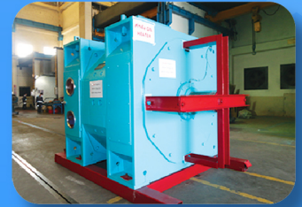
Rewinding DC Motor " HANGZHOU NEW HENGLI " 1,250 kW. 1,000 V. 1,358 A. 430/1,200 RPM.
