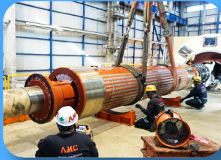
Generator " NISHISHIBA " 43,750 kVA. 11,000 V. 2,297 A. 1,500 RPM. 50Hz. WEIGHT 69,350Kg
